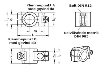
Adjustable clamp lever for d3 = GN 911-M 8-32 have to be ordred separately Adjustable clamp lever for d4 = GN 911-M 6-25 have to be ordred separately
